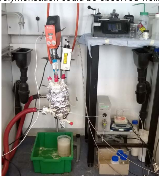
Figure 1. An image of the 500 mL reactor at UCAM during a semi-batch polymerization experiment, with an immersion Raman probe.
