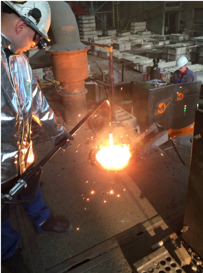
Figure 3: Photograph during hand lance temperature measurement using fibre optical sensor at foundry induction furnace
